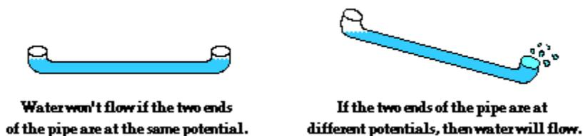
In conclusion, there are two requirements that must be met in order to establish an electric circuit. The requirements are
